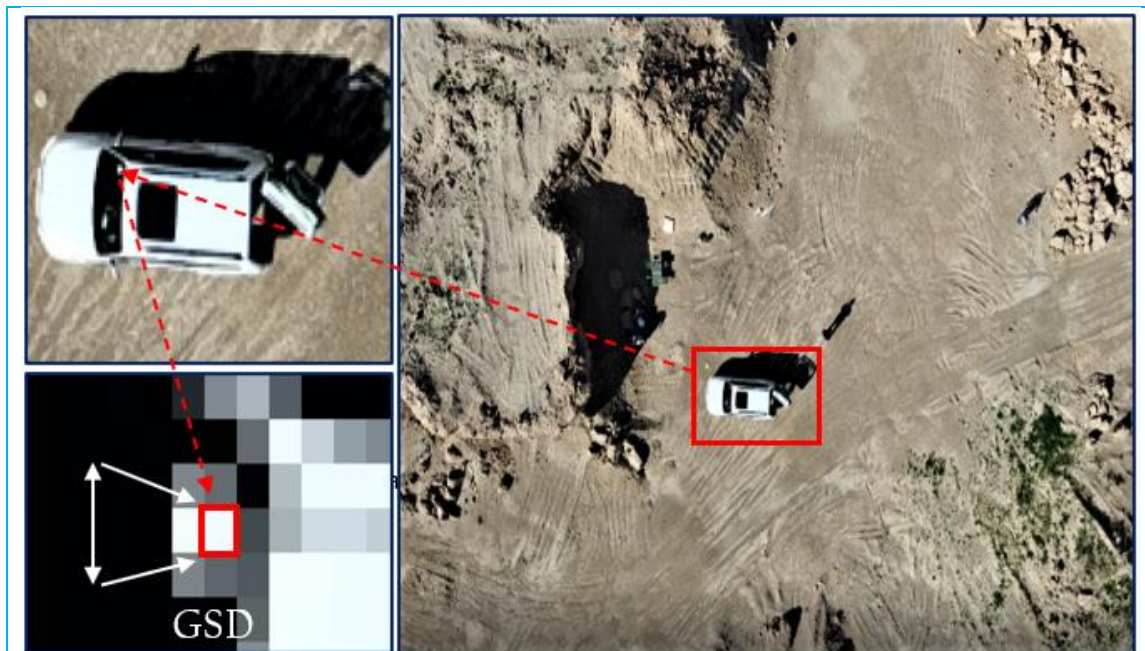
Fig.5: Calculation ground sampling distance
