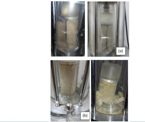
Fig. 2 Typical failure modes of treated specimens under uniaxial compression. (a) axial splitting (b) sh ear fracture
