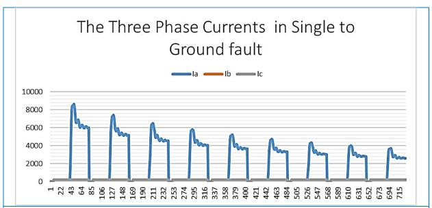
Fig.7 The Three Phase Currents in Single to Ground fault through nine cases along 200 Km between (Misan-Kut) station. (The x-axis indicates the NO. of data taken during the fault along 200 Km, y-axis indicates the values of the three-phase currents during the fault in different locations)
